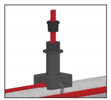
1. Insert cable without the braid through pipe standoff grommet as shown. Attach pipe standoff to pipe with pipe straps (Chromalox model PS not included). Leave braid outside of pipe standoff at grommet. For pipes smaller than 1 1/2" diameter a small pipe adapter (Chromalox model SPA not included) is required.
