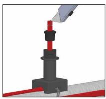
2. Score the outer insulation 1/2 inches from the end of cable. Lightly cut the outer jacket up the center to end of heating cable and remove the jacket from the cable.
