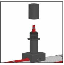
5. Slide end cap over cable. Grommet should be placed inside pipe standoff.
