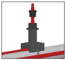
3. Using wire cutters trim exposed grounding braid away from the end of the cable.
